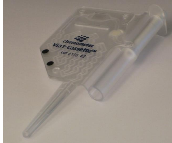
Figure 2 The Via1-Cassette. Here fluorescent dyes AO (Acridine Orange) and DAPI (4',6-diamidino-2-phenylindole) are immobilized in the first part of the flow system.
